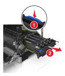
**8** Remove the used developer unit.
