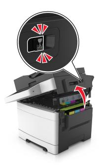
**2** Remove the toner cartridge by lifting the handle, and then gently pulling it away from the imaging kit.
