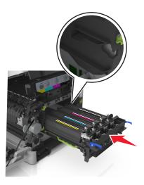
**15** Gently but firmly push the blue levers down until the imaging kit fits into place.
