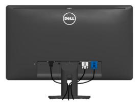
After attaching all necessary cables to your monitor and computer, (See Connecting Your Monitor for cable attachment), organize all cables as shown above.
