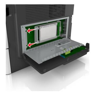
**c** Tighten the two screws.
