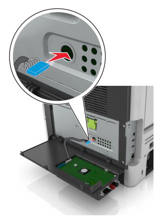
**11** Open the controller board shield using the green handle.
