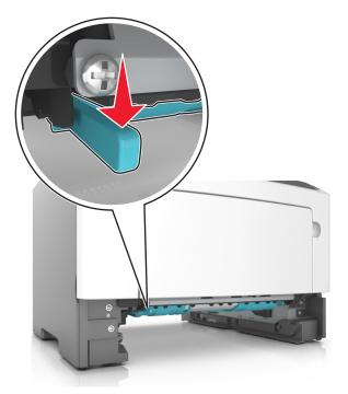
3 Firmly grasp the jammed paper on each side, and then gently pull it out.Note: Make sure all paper fragments are removed.
