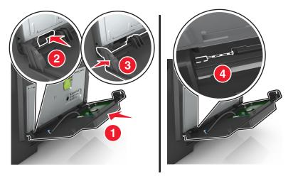
**10** Run the ISP cable through the controller board shield door.
