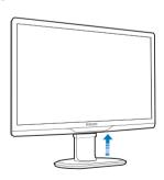
Place the monitor face down on a smooth surface, taking care to avoid scratching or damaging the screen. Then lift the monitor stand.
