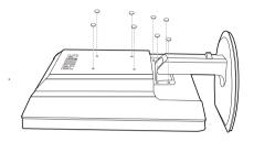
2. Remove the 4 screws and then remove the base from the monitor.
