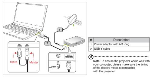
Connect the USB connector to your computer and plug the USB connector to the projector. If you want a brighter display, use power adapter or plug two USB connector to your computer.
