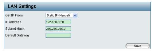
**IP Address:** The default IP address is **192.168.0.50**. Assign a static IP address that is within the IP address range of your network.
