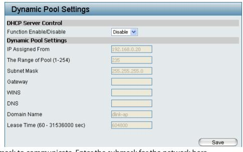
SubMask: All devices in the network must have the same subnet mask to communicate. Enter the submask for the network here.
