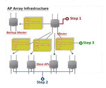
Up to eight stand-alone APs can be managed in an array. Members in the same AP Array group must be on the same subnet of the same model, and each AP is assigned with a unique IP address.
