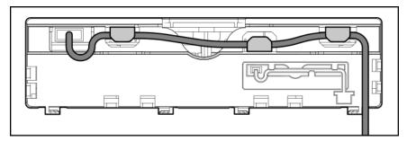
11. Install the Smart Storage Battery in the chassis:
