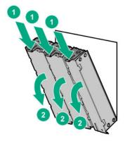
If the drive cage is to be installed in box 2 or 3, remove the drive cage blank. Retain the blank for future use.
