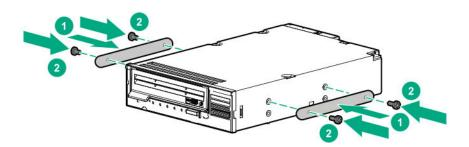
**13.** Slide the LTO tape drive into the half-height media bay 1 until the rear edge of the drive is aligned with the rear edge of the drive box.
