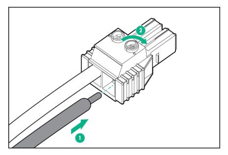
Install the terminal block connector in the power supply.
