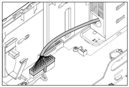
**12.** Remove the non-hot-plug power supply.
