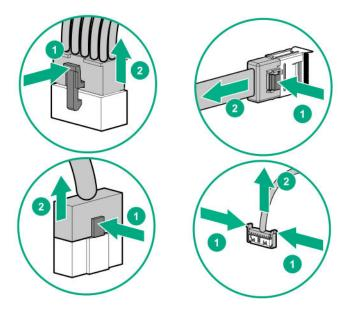
• Remove cables that are no longer being used. Retaining them inside the server can restrict airflow. If you intend to use the removed cables later, label and store them for future use.
