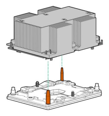
**CAUTION:** Be sure to tighten each heatsink nut fully in the order indicated. Otherwise, boot failure or intermittent shutdowns might occur.
