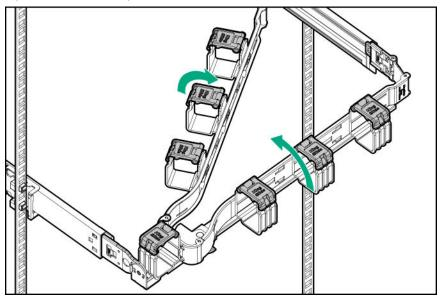
**4.** Route the rear panel cables and power cords though the CMA, and then close the cable clamps. Employ industry best practices in routing and managing these rear panel cables and power cords.
