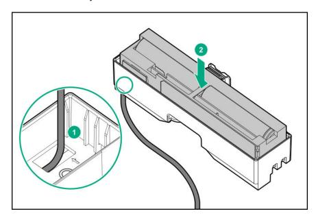
**10.** Secure the battery cable through the holder cable clips.
