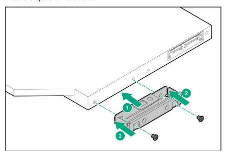
11. Install the optical drive in the drive cage.
