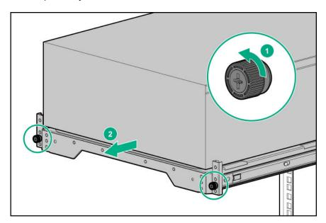
5. Remove the chassis rear bracket screws.
