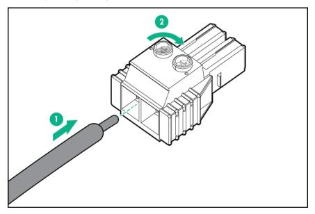
Insert the return wire into the right side of the connector, and then tighten the screw to 1.3 N m (10 lb-in) of torque.
