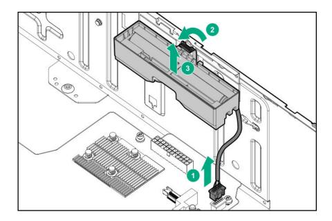
**11.** Disconnect the non-hot-plug power supply cable.
