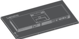
Step 4: Attach the mounting bracket from the VESA compatible wall mounting kit (100mm x100mm distance), VESA Mounting Screw M4 x 10 mm.
