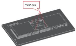
Step 5: Attach the LCD display to the wall, and follow the instructions in the wallmounting kit.
