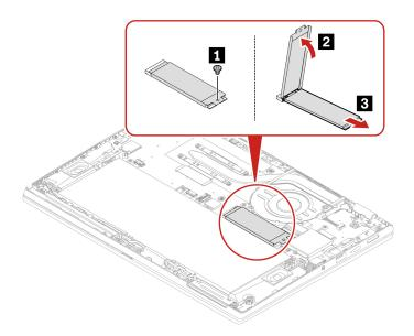
Step 2. Install the M.2 solid-state drive as shown below.
