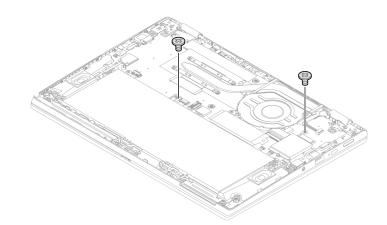
Step 5. Tighten the screws to secure the base cover assembly.
