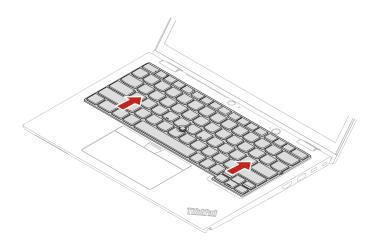
Step 3. Pivot the keyboard slightly upward 1 and then turn over the keyboard 2.
