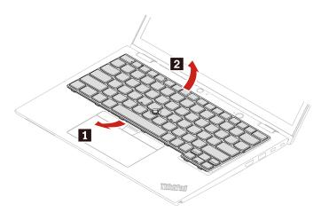
Step 4. Put the keyboard on the palm rest as shown and detach the connectors. Then, remove the keyboard.
