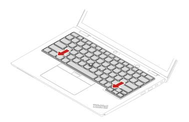
Step 4. Turn over the computer. Then, tighten the screws to secure the keyboard.
