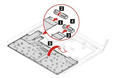
Step 2. Insert the keyboard into the keyboard bezel as shown. Ensure that the top edge of the keyboard (the edge that is close to the display) is under the keyboard bezel.
