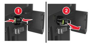
**3** Lift the staple guard, and then remove any jammed or loose staples.
