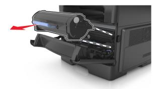
**3** Lift the blue handle, and then pull out the imaging unit from the printer.
