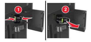
**3** Hold both sides of the empty staple case with your fingers, pull, and then lift the empty staple case from the cartridge.
