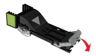
5 Insert staple cartridge back into the finisher until it *clicks* into place.
