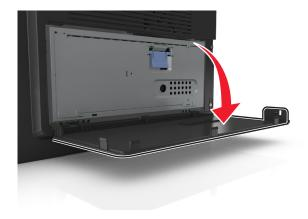
**2** Open the controller board shield using the blue handle.
