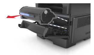
**3** Lift the blue handle, and then pull the imaging unit out of the printer.
