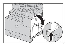
2 Hold and lower the tab to open the inner part.
