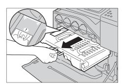
*8* Grasp the handles on the top of the transfer belt unit. Pull out the unit to remove it from the machine.
