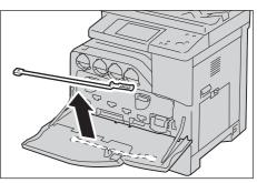
14 Remove the cleaning pad by pressing the amber gold tabs between your thumb and index finger.
