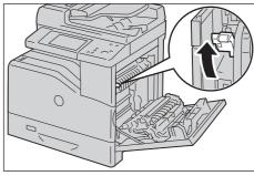
• To load envelopes using the optional Finisher-AB1, raise the lever as shown in the illustration.
