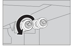
**4** Pull the separator roller hook out of the groove on the axle, and then slide the separator roller to the front.
