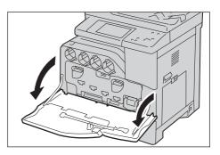
**2** Remove the cleaning rod from the backside of the front cover.
