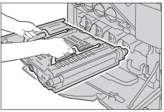
11 Align the arrows on the transfer belt unit with the arrows on the machine.
