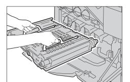
*13* Align the arrows on the transfer belt unit with the arrows on the machine.
