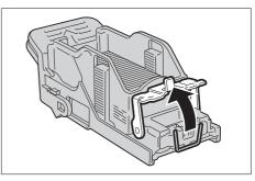
5 Remove the jammed staples (1), and then return the metal part pulled up in step 4 to the original position (2).
