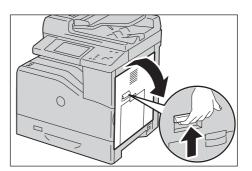
**4** Unlock the two levers on the transfer roller and lift up the roller to remove it.
