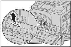
**7** Pull out the transfer belt unit until the line on the unit becomes completely visible.
