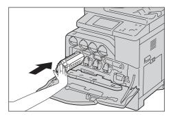
Remove the orange protective covering of the installed drum cartridge and discard it.
