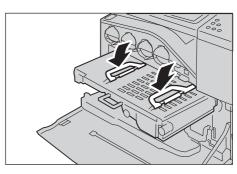
14 Push the front of the transfer belt unit to reinstall it in the machine until it stops.
