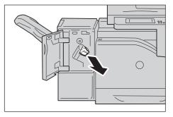
*3* After you take out the staple cartridge, check inside of the finisher for any remaining staples.
