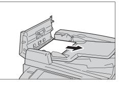
*3* If the massage on the screen instructs you to turn the knob, turn the knob to eject the document upward.
