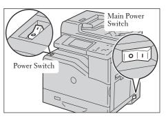
power off except when you connect a cable to the machine or clean the machine. Switching off the main power may erase the data in the memory when using the Fax service.
