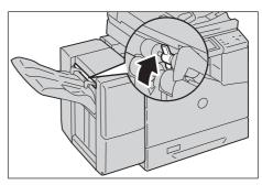
• To load print media other than envelopes using the optional Finisher-AB1, check if the lever is pulled down as shown in the illustration.
