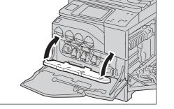
*18* Rotate the lock levers to secure the inner cover while pressing the cover with the other hand.
